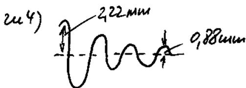
$\underline{\underline{\Lambda = \frac{1}{3} \ln \frac{222 \text{ mm}}{9,88 \text{ mm}} = 0,308}}$
