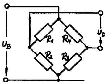
$$\frac{u_D}{u_B} = \frac{1}{4} \left( \frac{\Delta R_2}{R} + \frac{\Delta R_4}{R} - \frac{\Delta R_1}{R} - \frac{\Delta R_3}{R} \right)$$
