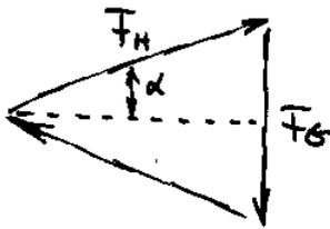
$\sin \alpha = \frac{FG/2}{FH} \Rightarrow \underline{\underline{FH = \frac{FG}{2 \cdot \sin \alpha}}}$  = m.f
