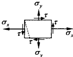
$$\sigma(\varphi) = \frac{\sigma_x + \sigma_y}{2} + \frac{\sigma_x - \sigma_y}{2} \cdot \cos(2\varphi) + \tau \cdot \sin(2\varphi)$$
