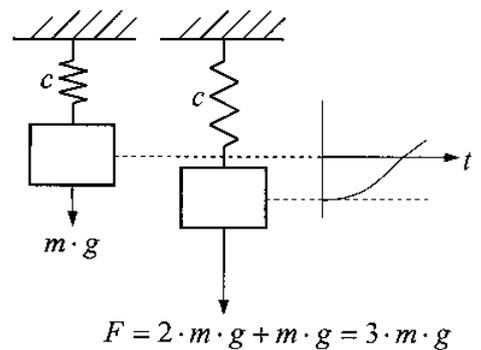
Geg.:  $m = 2 \text{ kg}; c = 20000 \text{ N/m}; g = 9,81 \text{ m/s}^2$
