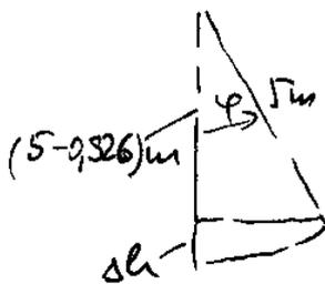
$$\cos \varphi = \frac{5 - 0,926}{5} \frac{\text{m}}{\text{m}} \Rightarrow \varphi = 35,4^\circ$$
