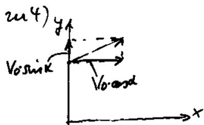
$$\dot{x}(t) = v_0 \cdot \cos \alpha = \text{Konst} \Rightarrow t = \frac{l}{v_0 \cdot \cos \alpha} \left( = \frac{26,21 \text{ m}}{20 \frac{\text{m}}{\text{s}} \cdot \cos 20^\circ} = 1,395 \text{ s} \right) \quad (1)$$
