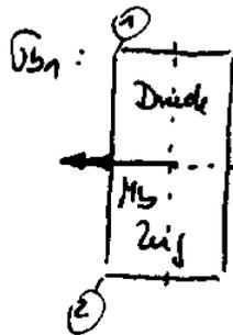
$\sigma_{\text{①}} = \frac{M_b}{W_b} = + \frac{10000 \text{ N} \cdot 25 \text{ mm}}{\frac{1}{6} \cdot 20 \cdot 50^2 \text{ mm}^3} = +30 \text{ N/mm}^2$
