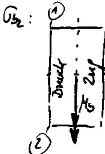
$\sigma_{\text{②}} = \sigma_{\text{①}} = - \frac{10000 \text{ N} \cdot 10 \text{ mm}}{\frac{1}{6} \cdot 50 \cdot 20^2 \text{ mm}^3} = -30 \text{ N/mm}^2$  (Druck)
