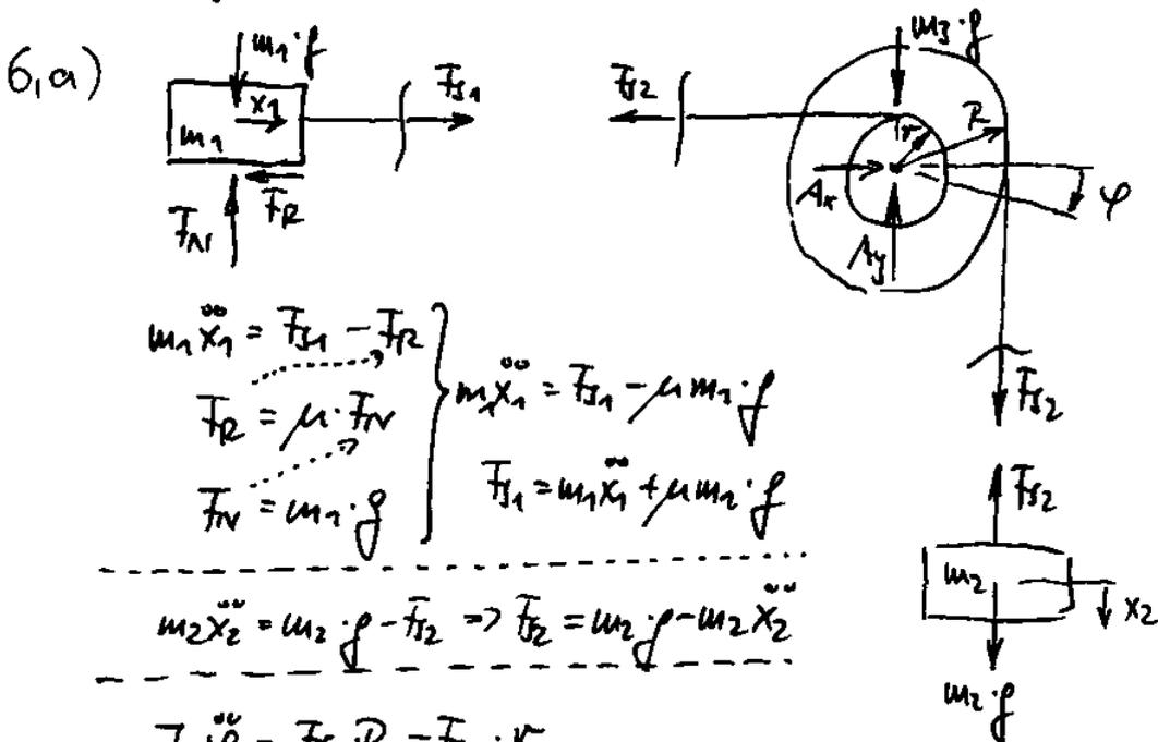
$$\left. \begin{aligned} m_1 \ddot{x}_1 &= F_{T1} - F_R \\ F_R &= \mu \cdot F_{N1} \\ F_{N1} &= m_1 \cdot g \end{aligned} \right\} \begin{aligned} m_1 \ddot{x}_1 &= F_{T1} - \mu m_1 g \\ F_{T1} &= m_1 \ddot{x}_1 + \mu m_1 g \end{aligned}$$
