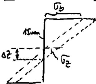
$$\frac{\sigma_b}{15 \text{ mm}} = \frac{\sigma_z}{\Delta z} \Rightarrow \Delta z = \frac{\sigma_z}{\sigma_b} \cdot 15 \text{ mm} = \frac{2,946}{128,56} \cdot 15 \text{ mm} = 0,344 \text{ mm}$$
