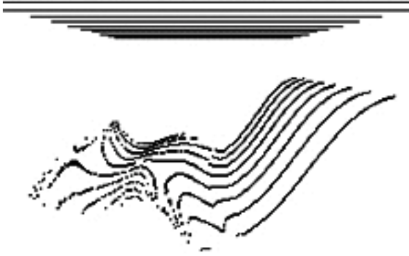
Figure 6: Highlight lines indicating a C^1 blend
